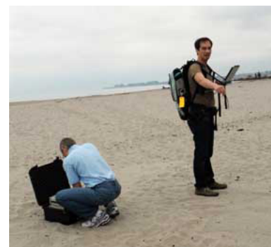
Brad Lobitz (CSUMB) and George Scheer (UCD) use a field spectroradiometer to gather ground truth data at Rio Del Mar beach.
