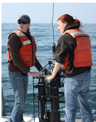
Above: Misty Blakely and Anna McGaraghan (UCSC) prepare to launch an optical instrument package measuring hyperspectral scattering and absorption as well as salinity, temperature, and depth from the R/V John Martin in Monterey Bay during COAST. Below: Mike Jacox (UCSC) uses a handheld sunphotometer to measure aerosol optical depth and water vapor at the air-sea interface.
