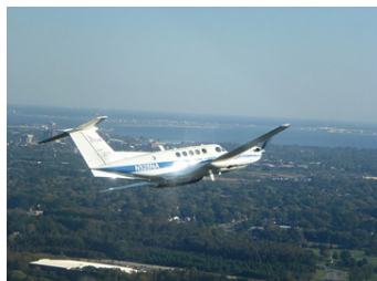
The NASA Langley UC-12 aircraft served as the remote sensing platform during DEVOTE, which carried the HSRL and the RSP.
